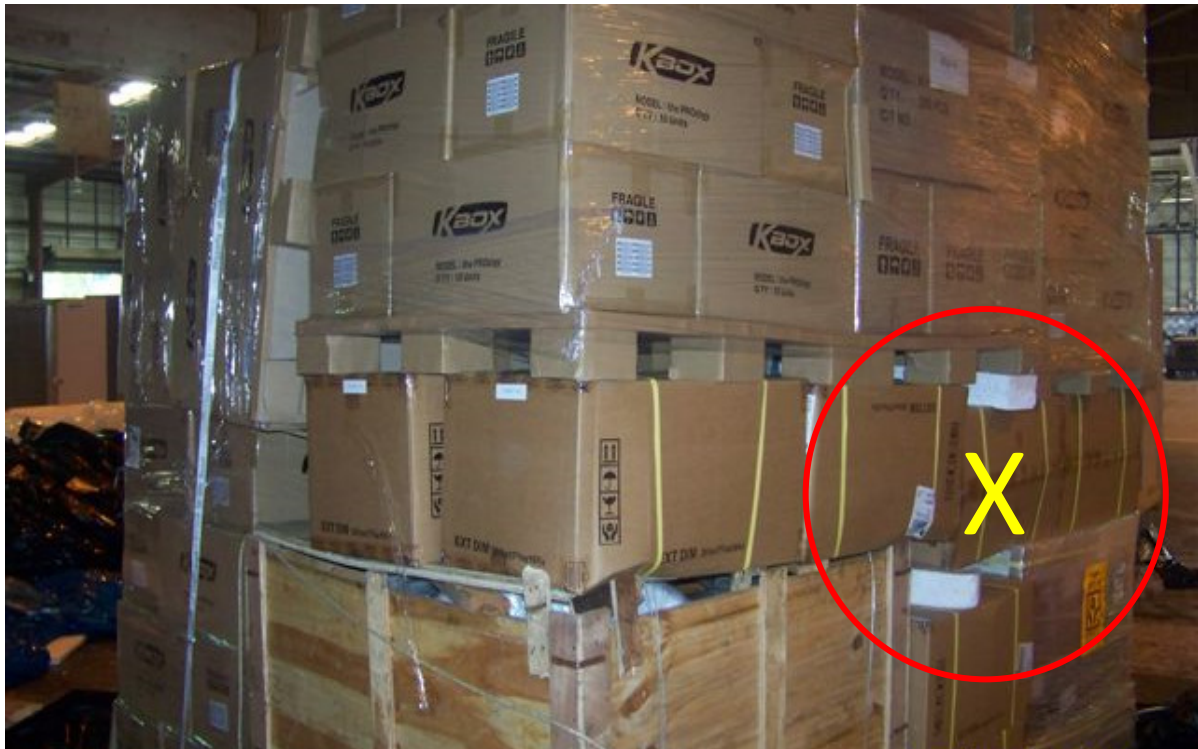
Example E: Styrofoam board is for weight support and level purpose ( Reject )
