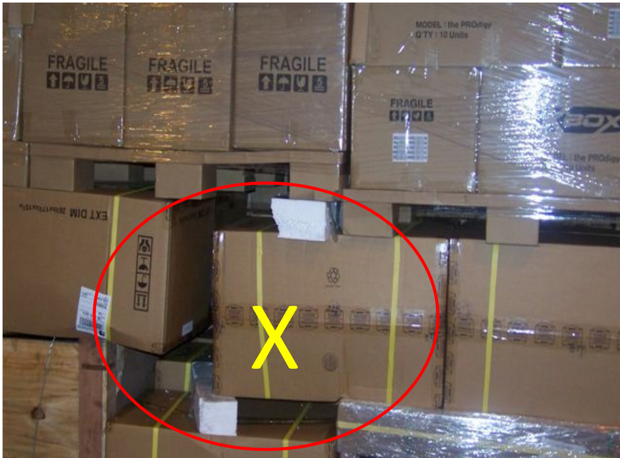
Example F: Styrofoam board is for weight support and level purpose plus one piece loaded upside down ( Reject )
